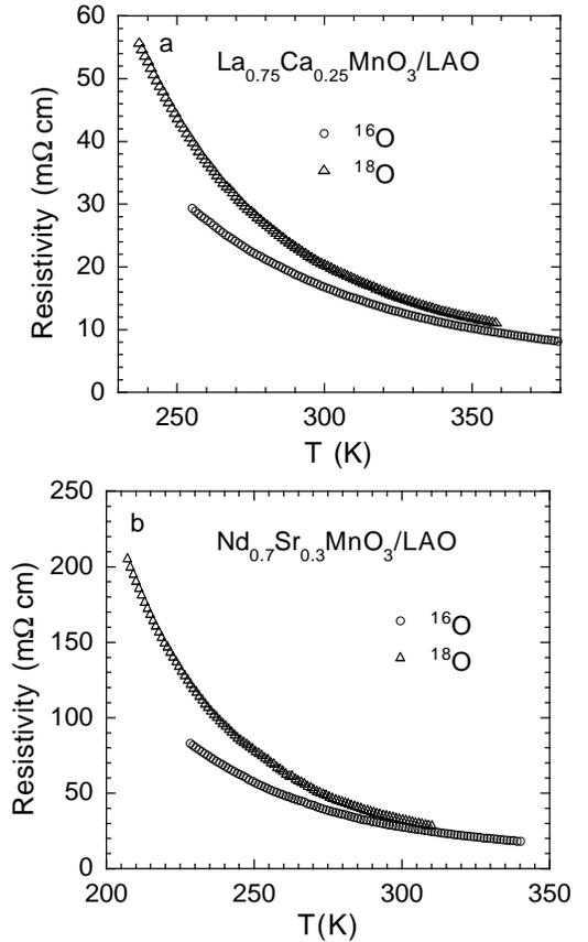
FIG. 1. The temperature dependence of the resistivity of the oxygen-isotope exchanged films of a)  $\text{La}_{0.75}\text{Ca}_{0.25}\text{MnO}_3$  and b)  $\text{Nd}_{0.7}\text{Sr}_{0.3}\text{MnO}_3$ . The data are the same as those reported in Ref. [2].
