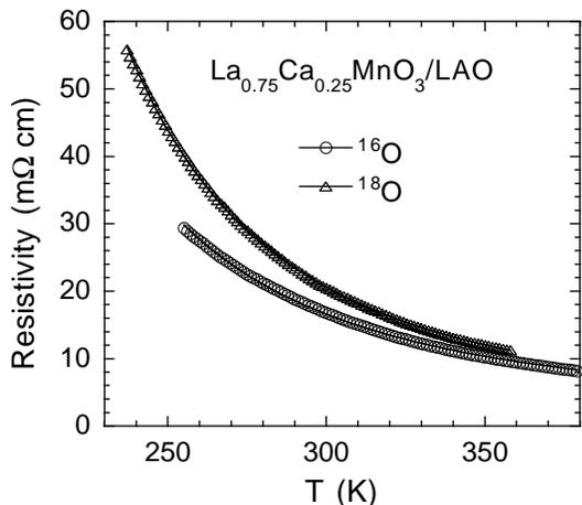
FIG. 3. The temperature dependence of the resistivity of the oxygen-isotope exchanged films of  $\text{La}_{0.75}\text{Ca}_{0.25}\text{MnO}_3$ . The solid lines are the curves best fitted by Eq. 6. The fitting parameter  $B$  for the  $^{16}\text{O}$  sample is larger than that for the  $^{18}\text{O}$  sample by 27%.
