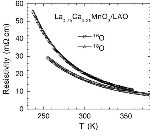
FIG. 2. The temperature dependence of the resistivity of the oxygen-isotope exchanged films of  $\text{La}_{0.75}\text{Ca}_{0.25}\text{MnO}_3$ . The solid lines are the curves best fitted by Eq. 1. The fitting parameter  $D$  for the  $^{16}\text{O}$  sample is larger than that for the  $^{18}\text{O}$  sample by 20%.
