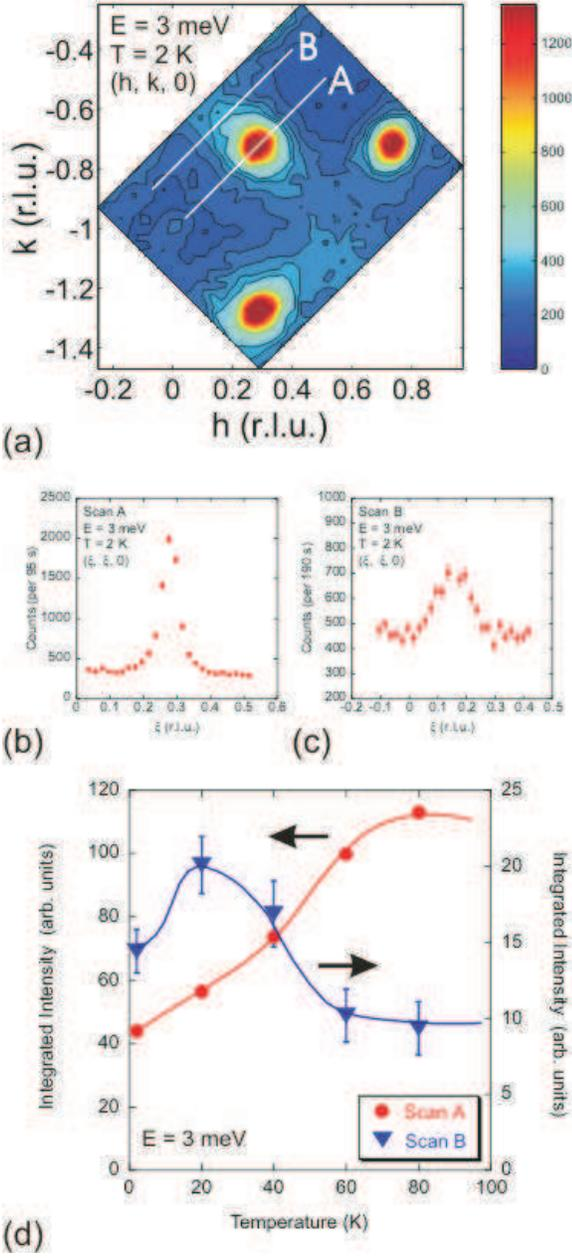
FIG. 7: (Color online) Low energy scattering from  $\text{La}_{3/2}\text{Sr}_{1/2}\text{NiO}_4$  measured on IN8 at an energy of 3 meV and a temperature of 2 K. (a) Map of the scattering intensity in the  $(h, k, 0)$  reciprocal lattice plane. (b) and (c) Cuts along the lines marked A and B in (a). (d) Temperature dependence of the integrated intensity of the peaks shown in (b) and (c). The lines are guides to the eye.
