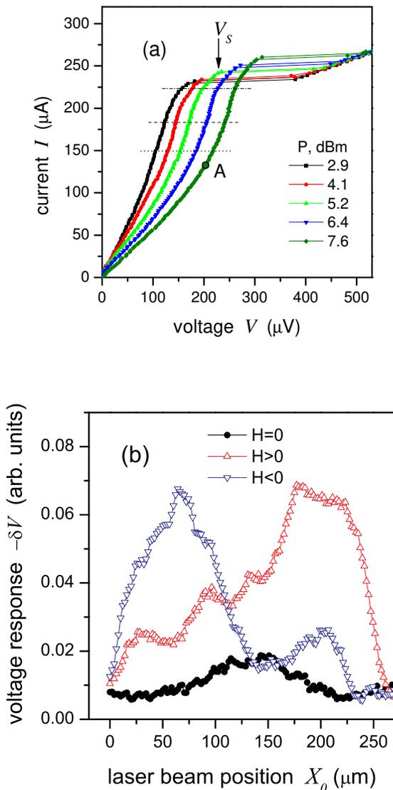
FIG. 3: (a)  $I$ - $V$  curves for different power levels obtained at the same regime as ones from Fig. 1(b) but at higher temperature  $T = 5$  K; (b) LSM response of the junction in a state corresponding to the marked bias point A in (a), at zero (solid circles) and non-zero dc magnetic fields ( $H = 2.3$  Oe up triangles,  $H = -2.3$  Oe down triangles).
