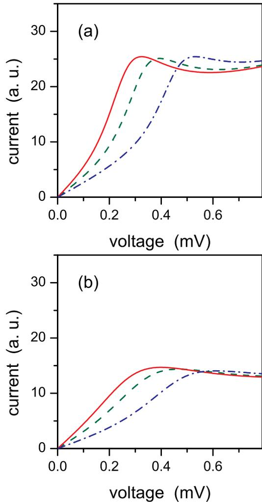
FIG. 7: The power dependence of  $I$ - $V$  curves calculated using Eq. (7) for two values of parameter  $\delta$ : (a)  $\delta = 0.0001$ ; (b)  $\delta = 0.0002$ . The power levels correspond to  $P = 2, 5, 7$  dBm. In both cases the linear slope corresponding to quasiparticle resistance  $R = 50$  k $\Omega$  (a) and  $R = 140$  k $\Omega$  (b), is added.
