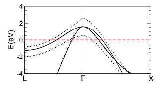
FIG. 1: LDA band-structure of diamond with x=0.1 holes/C (full lines). A frozen optical zone-center phonon with two bonds stretched and two contracted by  $u/\sqrt{2}$  splits the bands by  $\pm Du$  (dotted lines). u=0.05Å.
