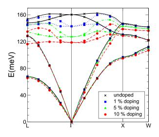
FIG. 2: Phonon dispersions calculated with the linear-response method for diamond with x = 0, 1, 5, and 10 % hole doping.
