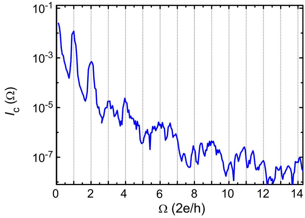
FIG. 4. Fourier transform of the SQUID-oscillations shown in Fig. 3(a).
