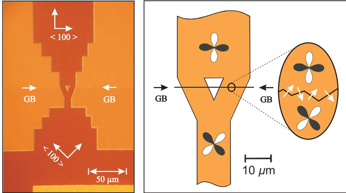
FIG. 2. Micrograph (left) and sketch (right) of a  $\text{YBa}_2\text{Cu}_3\text{O}_{7-\delta}$  SQUID used in the study. The grain boundary is marked by the arrows labelled 'GB'. The blow-up on the right sketches the facet structure and the corresponding Josephson current crossing the boundary.
