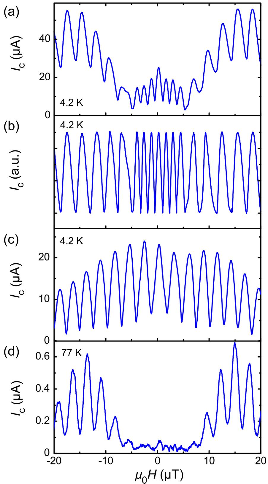
FIG. 3. (a) Magnetic field dependence of the critical current of a  $\text{YBa}_2\text{Cu}_3\text{O}_{7-\delta}$  SQUID with an asymmetric  $45^\circ$  grain boundary measured at 4.2 K; (b) same data as (a) with the oscillation amplitude numerically normalized; (c) field dependence of the critical current of a control SQUID with a symmetric  $45^\circ$  boundary; (d) same as (a), but measured at 77 K.
