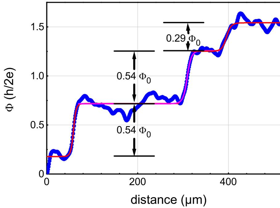
FIG. 1. Magnetic flux  $\Phi$  generated at 4.2K by a (110)/(100) grain boundary in a  $\text{YBa}_2\text{Cu}_3\text{O}_{7-\delta}$ -film, measured by scanning SQUID microscopy.
