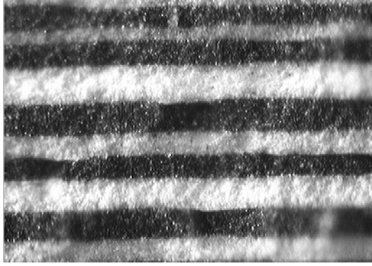
Fig.1. Fragment of cross-section of multilayer structure NFO1-PZT # 3.
