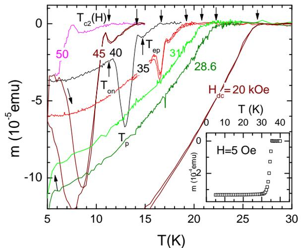
FIG. 1: Zero field and field cooled temperature variation of the global magnetic moment of MgB<sub>1.96</sub>C<sub>0.04</sub> crystal for  $\mathbf{H} \parallel c$ -axis. The inset shows the temperature variation of the magnetic moment for  $H = 5$  Oe. The small positive peak at the region of  $T_{ep}$  is an artifact due to field inhomogeneity.
