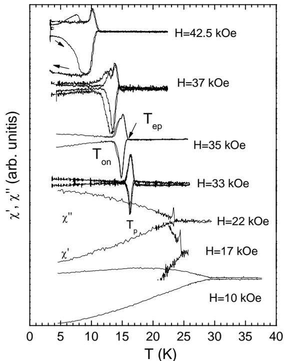
FIG. 2: Real ( $\chi'$ ) and imaginary ( $\chi''$ ) local fundamental ac-susceptibility as a function of temperature, for  $H_{ac} = 8.8$  Oe and ( $H_{dc} = 10 - 42.5$  kOe). For  $H > 20$  kOe the peak effect is always observed.
