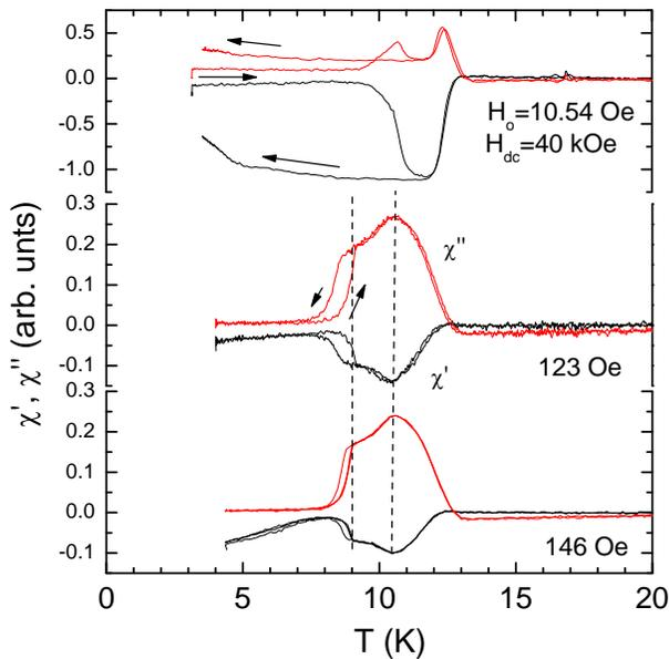
FIG. 3: Dependence of the hysteretic local ac-susceptibility for  $H_{dc} = 40$  kOe and for various amplitudes of the ac-field.
