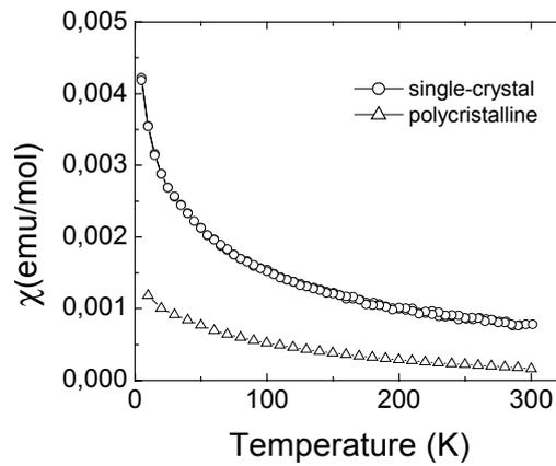
Fig 5: Temperature dependence of the magnetic susceptibility along the ab-plane of a single crystal (circles), and in a polycrystalline sample (triangles).
