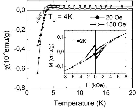
Fig.7: Magnetization curves in FC-ZFC of  $\text{Na}_x\text{CoO}_2.n\text{H}_2\text{O}$  at 20 Oe and 150 Oe. The  $T_C$  is 4 K. Inset: Magnetization vs. field hysteresis loop taken at 2 K.
