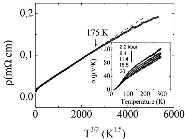
Fig.1: Temperature dependence of the resistivity along the ab-plane versus  $T^{3/2}$ , and thermoelectric power under pressure of a dense polycrystalline sample (inset).
