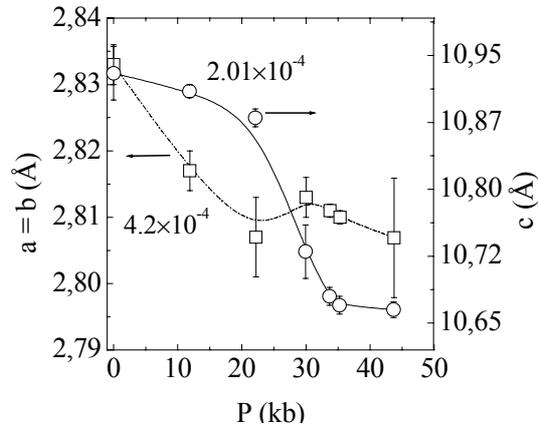
Fig. 2: Pressure dependence of the room temperature lattice parameters obtained in a powder from crushed single crystals. The numbers indicate the compressibility in the ab-plane and along the c-axis, up to 20 kbar. Lines are guides to the eye.
