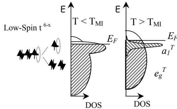
Fig.4: Schematic band diagram of the system  $\text{Na}_x\text{CoO}_2$ . The dotted circle represents a hole introduced by  $\text{Mn}^{4+}$ .  $T_{\text{MI}}$  is the temperature at which the resistivity becomes thermally activated.
