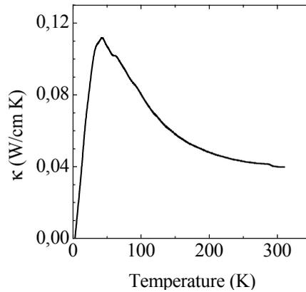
Fig.6: Temperature dependence of the lattice thermal conductivity of a cold-press sintered polycrystalline sample.
