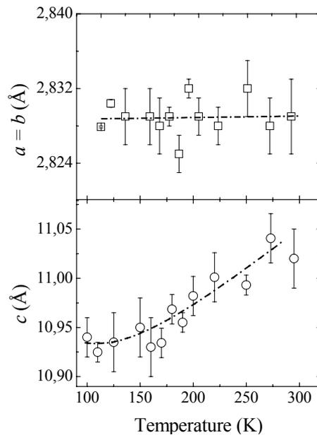
Fig.3: Thermal evolution of the in-plane (above) and along the c-axis (below) lattice parameters of a polycrystalline sample. Si was used as an internal standard. Lines are guides to the eye.
