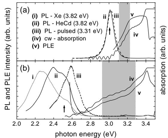
FIG. 1. Room temperature cw-PL using a Xe lamp source at 325 nm (i) and a HeCd laser (ii); time-integrated, below  $I_{th}$ , pulsed-PL (iii), Cw-absorption (iv), and PLE (v) for the (a) 12%, and (b) 23% MQW samples. The shaded regions show the states between the barrier and QW band edges. Arrows show the detection energies for the PLE.
