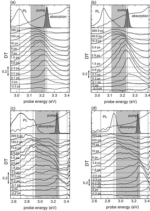
FIG. 3. SR-TRDT for (a) below ( $60 \mu\text{J}/\text{cm}^2$ ) and (b) above ( $160 \mu\text{J}/\text{cm}^2$ )  $I_{th}$  (12%), and (c) below ( $150 \mu\text{J}/\text{cm}^2$ ) and (d) above ( $380 \mu\text{J}/\text{cm}^2$ )  $I_{th}$  (23%). Shaded regions show the states between the barrier and the QW band edges.
