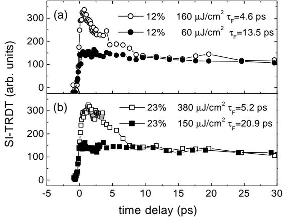
FIG. 2. SI-TRDT for the (a) 12% and (b) 23% MQW samples, excited at energies near the barrier band edge for densities above (open) and below (filled)  $I_{th}$ . Spectral integration occurred from the GaN band edge (3.40 eV) to below the In-GaN QWs (2.92 and 2.55 eV for the 12% and 23% samples, respectively).
