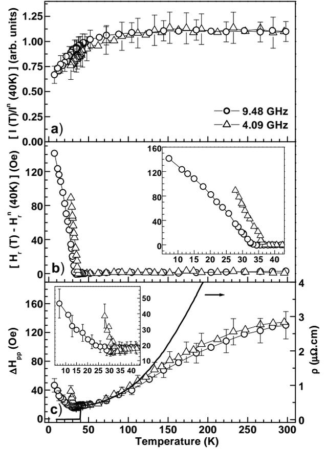
FIG. 3. X and S-band  $T$ -dependence of the: a) relative CESR intensity,  $I(T)/I^n(40\text{ K})$ , b) shift of the resonance field,  $H_r(T) - H_r^n(40\text{ K})$ , and c) linewidth,  $\Delta H_{pp}(T)$ , and resistivity,  $\rho(T)$ , from ref. [20].
