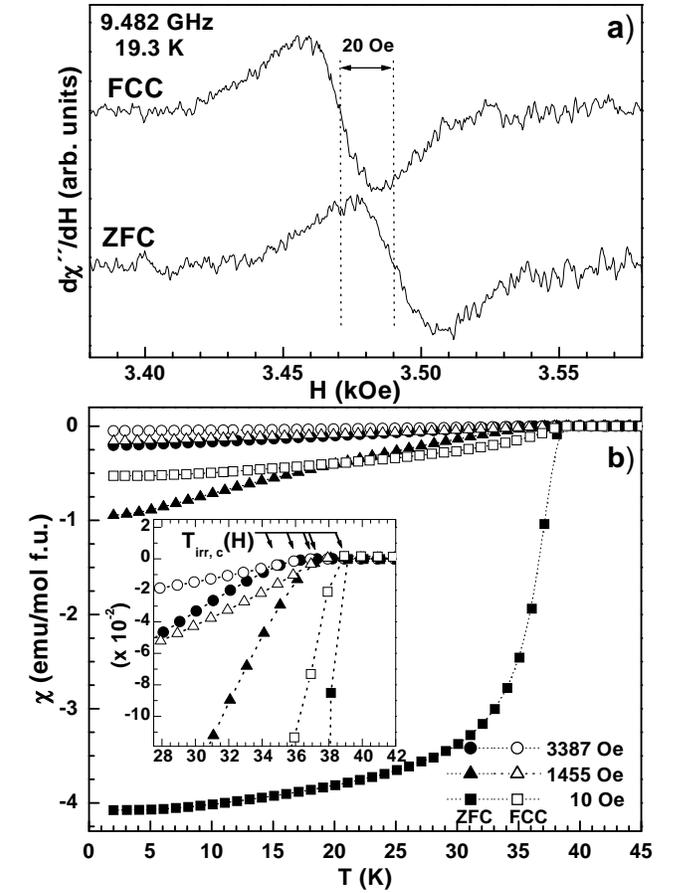
FIG. 2. a) FCC and ZFC X-band CESR spectra at 19.3 K, b)  $T$ -dependence of the FCC and ZFC  $dc$ -magnetic susceptibility of  $\text{MgB}_2$  for  $H = 10$  Oe, 1455 Oe and 3387 Oe.
