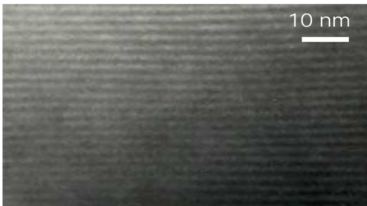
Figure 1. TEM image of a digital alloy with a repeat unit of Mn (0.5 ML)/GaSb (12 ML). The dark lines correspond to Mn-containing layers.
