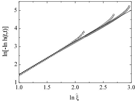
FIG. 1: Plot of  $\ln[-\ln h(\ell, t)]$  versus  $\ln \hat{\xi}$  for the two-dimensional incipient percolation cluster. The radii of the absorbing “circular” boundaries are  $\ell = 40$  (triangles),  $\ell = 100$  (circles) and  $\ell = 160$  (squares). The line represents the function  $h(\ell, t) = \hat{A} \hat{\xi}^{-\hat{\mu}\hat{v}} \exp(-\hat{c}\hat{\xi}^{\hat{v}})$  with  $\hat{A} = 1$ ,  $\hat{\mu} = -0.4$ ,  $\hat{c} = 0.9$  and  $\hat{v} = d_w^\ell / (d_w^\ell - 1) = 1.714$ .
