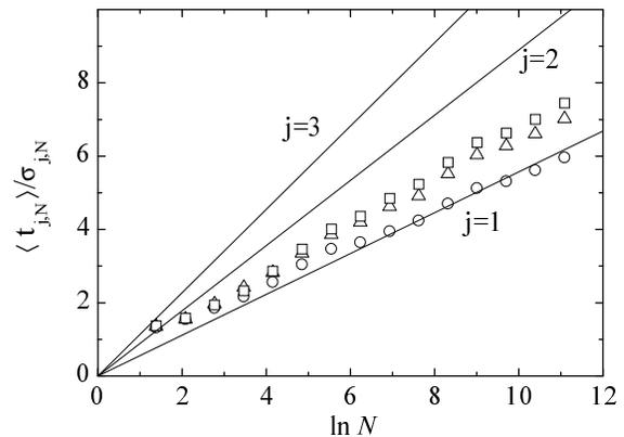
FIG. 6: Plot of  $\langle t_{j,N} \rangle / \sigma_{j,N}$  versus  $\ln N$  for the two-dimensional incipient percolation aggregate with  $\ell = 50$ . The circles, triangles and squares denote the simulation results for  $j = 1, 2$  and  $3$ , respectively. The lines are the theoretical predictions with  $d_w^\ell = 2.4$  and  $\hat{v} = d_w^\ell / (d_w^\ell - 1) = 1.714$ .
