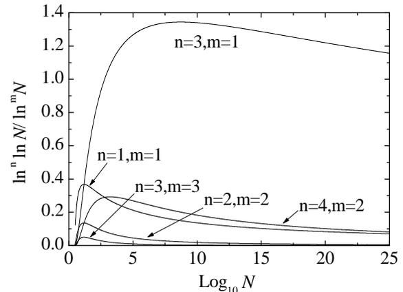
FIG. 7: Plot of  $\ln^n \ln N / \ln^m N$  versus the decimal logarithm  $\text{Log}_{10} N$  for several pairs  $(n, m)$ . These functions gauge the relative error of different finite-order asymptotic approximations to the order-statistics quantities.
