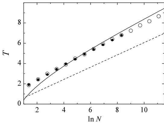
FIG. 8: Plot of  $T = [\langle t_{1,N} \rangle / r^{d_w}]^{-\delta}$  versus  $\ln N$  for the two-dimensional incipient percolation aggregate, where  $N = 2^2, 2^3, \dots, 2^{16}$  and  $\delta = 1/(d_w - 1)$ . The filled [hollow] circles are the simulation results for  $r = 50$  [ $r = 75$ ]. The broken and solid lines are the zeroth-order and first-order asymptotic approximations, respectively, with  $\tilde{c} = 1.65$ ,  $\tilde{v} = 1.56$  and  $\tilde{\mu} = -1.85$ .
