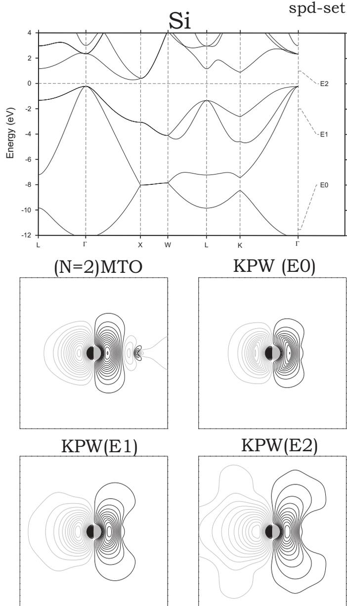
Figure 1: Band structure of Si calculated with the Si *spd*-QMTO basis set corresponding to the energy mesh shown on the right-hand side (solid lines). The contour plots show the Si  $p$  orbital pointing in the  $[111]$ -direction between two nearest neighbors in the  $(2\bar{1}\bar{1})$ -plane. Shown are the kinked partial waves (KPWs) at the three energies and the QMTO. The KPWs are normalized to 1, times a cubic harmonics, at the central hard sphere. The contours are the same in all plots.
