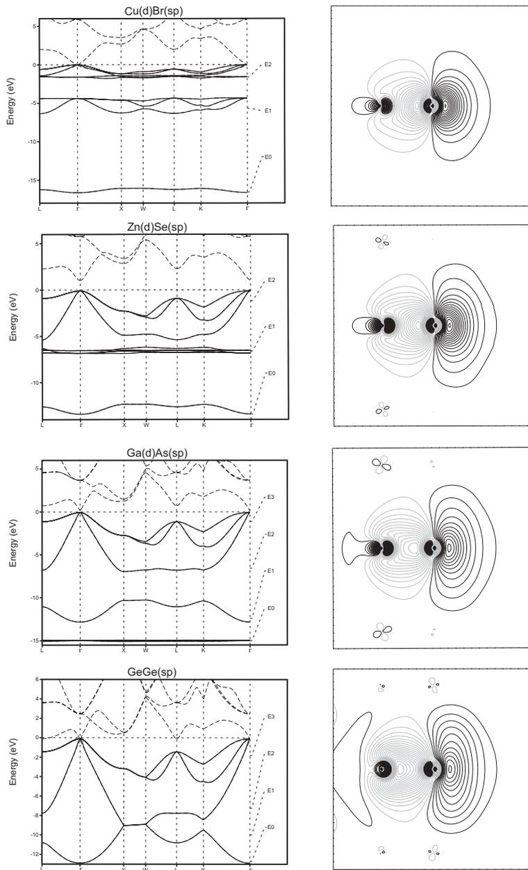
Figure 5: Valence bands (solid lines) of the series CuBr – Ge, calculated with the ionic basis sets where the *sp*-MTOs are on the anion and, except for Ge, the *d*-MTOs are on the cation. The exact bands are given by dashed lines. The contour plots show the  $p_{111}$ -MTO on the anion (the atom to the right). The ionicity decreases and the covalency increases from the top to the bottom.
