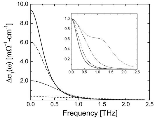
FIG. 1.  $\Delta\sigma_1$  as a function of frequency ( $\omega/2\pi$ ) for anticorrelated variations in  $\rho_s$  and  $\rho_n$ . Spectral weight decreases for increasing  $v_s q \tau$ : 0.25, 0.5, 1.0, and 2.0. The same curves are shown in a normalized plot in the inset.
