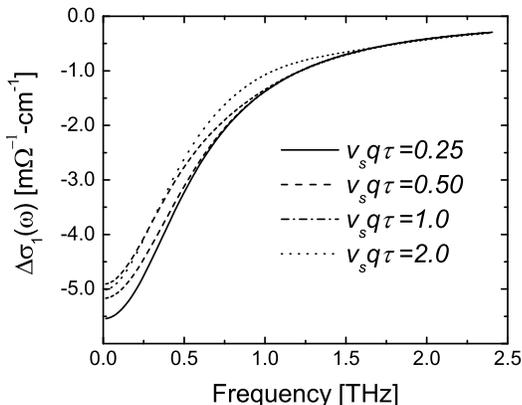
FIG. 3.  $\Delta\sigma_1$  vs. frequency for the same parameters as Fig. 1, except variations in  $\rho_s$  and  $\rho_n$  are positively correlated.
