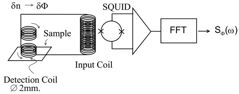
Fig. 1. Experimental configuration: an astatic coil is mounted over the sample to detect magnetic flux noise fluctuations. A DC SQUID amplifies the fluctuations which are then fed into the FFT.
