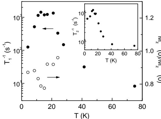
FIG. 4.  $^{139}\text{La}$  spin-lattice relaxation rate vs.  $T$ . Closed circles – fast contribution, open circles – relative value of the fast contribution (scale on the right).  $T_1$  (slow) is of the order of 0.1 s. Inset:  $^{139}\text{La}$  spin-spin dephasing rate vs.  $T$ .
