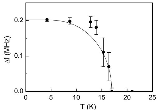
FIG. 3.  $^{139}\text{La}$  NQR line 1 splitting for  $m = 7/2$  vs.  $T$ . Drawn line is the mean field staggered magnetization for  $S=1/2$  ( $T_N=17$  K,  $\Delta f(0)=202$  kHz).
