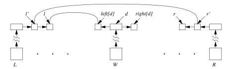
Here the square box above L represents the data structure node corresponding to the word L. This points to a list of disjuncts, each of which is shown as a rectangular box above the word. The disjunct in turn points to two linked lists of connectors, shown here as small square boxes.
