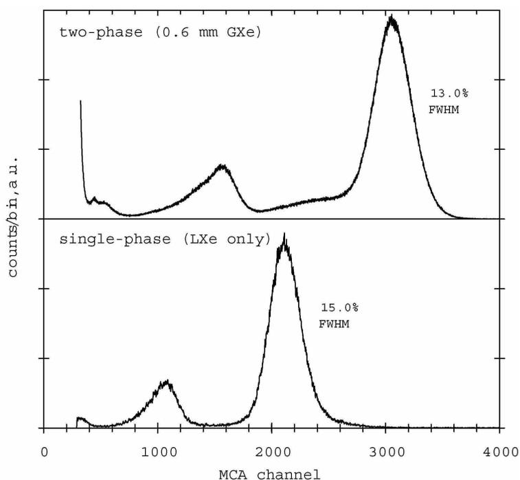
Fig. 15. Pulse height spectra obtained from the  $^{241}\text{Am}$  primary scintillation signals during the first cool-down test. The two panels correspond to two different liquid xenon levels. The highest energy peaks in both spectra are at 59.6 keV.
