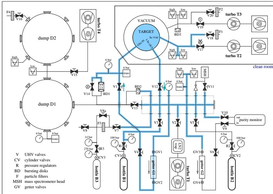
Fig. 12. Schematic diagram of the gas purification system.
