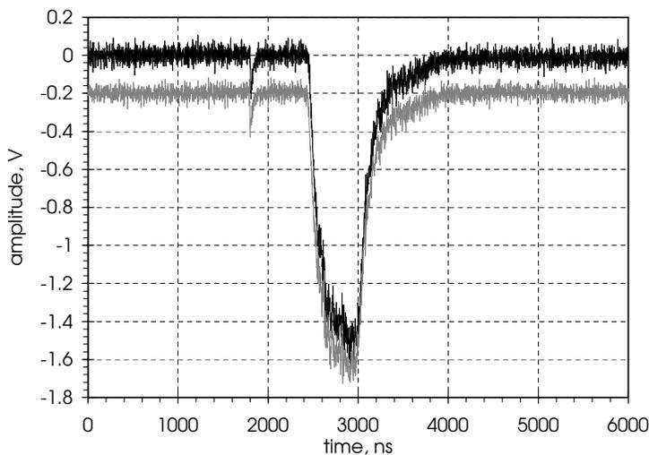
Fig. 17. Summed waveforms from a  $\gamma$ -ray event showing a fast primary pulse followed by the secondary wider pulse from electroluminescence in the gas phase caused by ionisation drifted from the event site. The two traces shown are from the dual range DAQ. The low-sensitivity data have been multiplied by 10.
