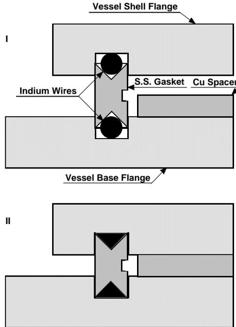
Fig. 8. Vacuum seal between the cylindrical wall section and the bottom flange before (I) and after (II) sealing.
