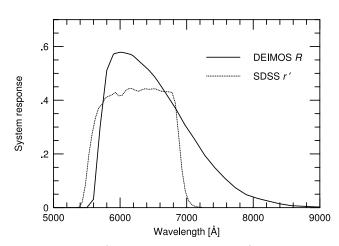
FIG. 1.— System (telescope, filter, and detector) response curves of R band filter used in the DEIMOS imaging (solid line) and the SDSS r' filter (dotted line). The r' filter is part of the system devised to calibrate the SDSS survey (Smith et al. 2002), and is shown here to illustrate the differences in bandpass of the filters. Note that in the actual calibration of the TKRS catalogue, the r-band data from the SDSS DR1 release were used.
