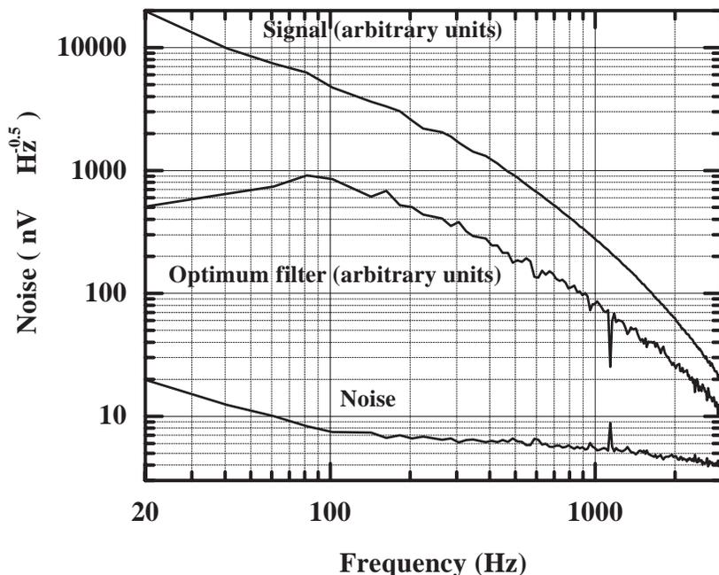
FIG. 9.—Total noise spectrum from a typical pixel, along with the X-ray pulse power spectrum and the resulting optimum filter response.
