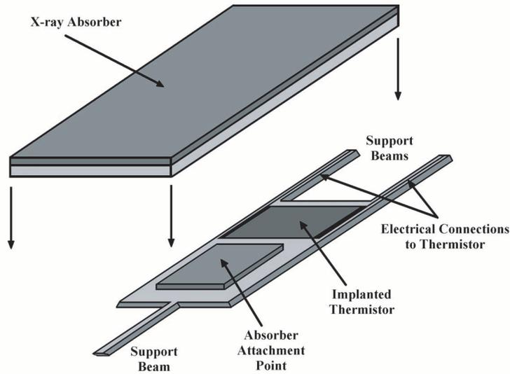
FIG. 3.—Detector pixel assembly. The HgTe X-ray absorber on a  $14 \mu\text{m}$  silicon substrate is attached to the small silicon spacer and the spacer to the pixel body with epoxy. Dimensions are given in Table 1.
