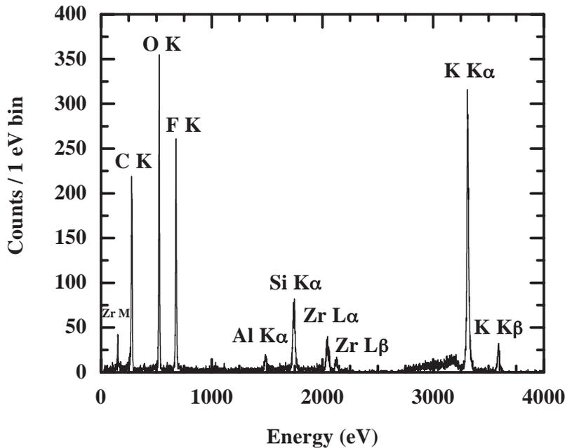
FIG. 11.—Calibration source spectrum taken during the 30 minutes immediately before launch. These lines are used to establish the energy scale, which is well fit by a cubic polynomial.
