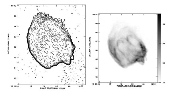
Fig. 2.— The supernova remnant W49B at 327 MHz. The sub-milliJansky sensitivity of this image makes it one of the highest dynamic range, low-frequency images ever obtained by the VLA. (a) The rms noise level in the image is  $0.62 \text{ mJy beam}^{-1}$ , and the contour levels are  $0.62 \text{ mJy beam}^{-1} \times -3$ , 4, 5, 7.07, 10, 14.1, 20, . . . . The beam is  $6.6 \times 6.2 \times 6.2$
