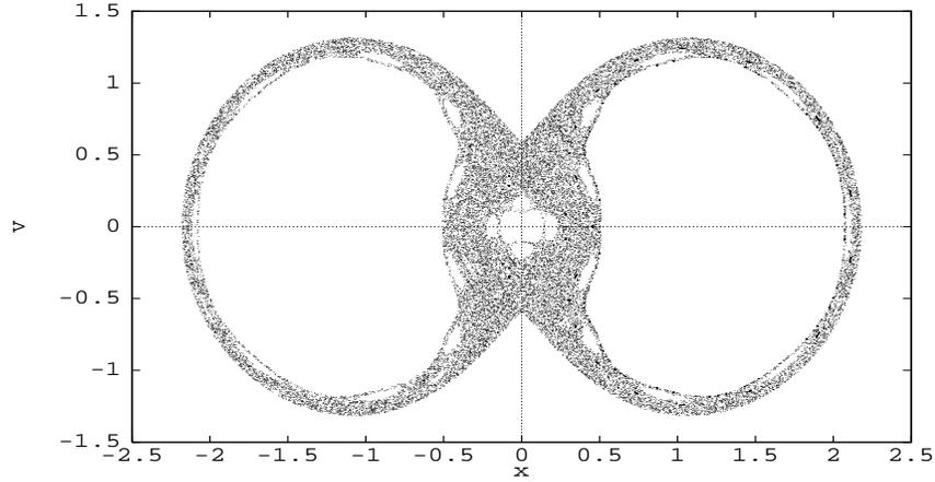
Figure 1: Stroboscopic plot of the chaotic sea in the core-halo model. Snapshots were taken at successive beam minima for 32 test particles. Parameter values were  $r(0) = 0.6$ ,  $\dot{r}(0) = 0$ , and  $\eta = 0.2$ .
