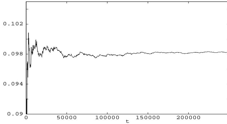
Figure 3: (a) Positive Lyapunov exponent for the van der Pol oscillator with parameters  $\lambda = -5$ ,  $a = 5$ , and  $\omega = 2.466$  (taken from Ref. [4]). The simulation was run for  $10^5$  periods of the driving force using 100 million time steps for Eqns. (18) and 200 million time steps for the fiducial trajectory. The integrators were third-order Runge-Kutta and fourth-order symplectic, respectively.
