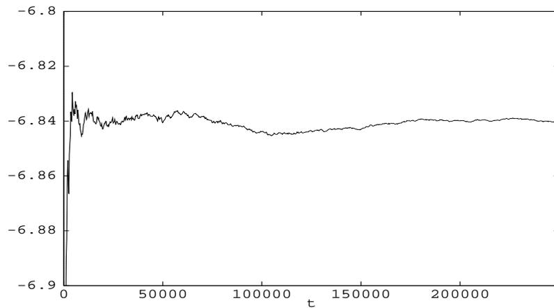
Figure 3: (b) Negative Lyapunov exponent for the van der Pol oscillator with the same parameters as in Fig. 3(a).
